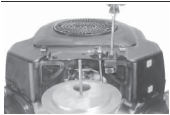
Figure 9-15. Removing Control Panel.
